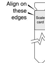
Align the self-adhesive printed scale card onto the flexible strip and insert the strip into the indicator as shown above.
