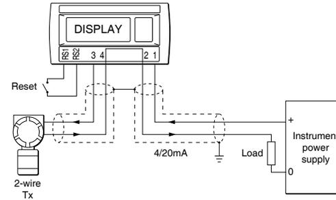
Fig 3 Typical measurement loop
