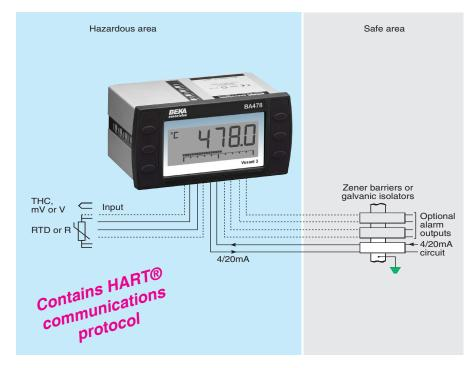
The new BA478C is a second generation panel mounting intrinsically safe loop powered indicating temperature transmitter which replaces the BA378C. It provides an accurate local digital temperature display, plus a 4/20mA output that may be scaled to represent any temperature range. Although incorporating new facilities such as HART® digital communication, diagnostics and a robust enclosure with an IP66 front, the BA478C remains electrically and mechanically compatible with the earlier model.
