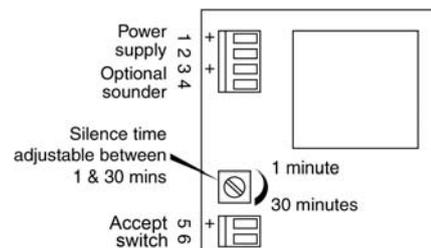
When the beacon is used alone i.e. without a sounder, terminals 5 & 6 should be connected together
