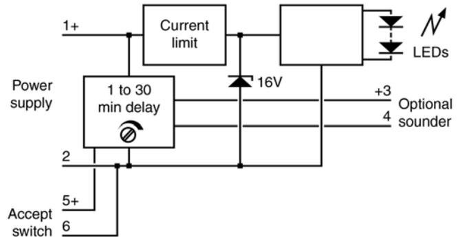
Fig 1 Simplified block diagram
