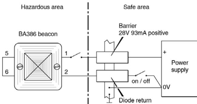
Fig 5 Single stage alarm using two channel barrier.
