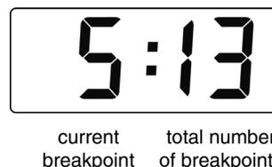
Increasing the number of segments will provide a more accurate approximation of the flowmeter characteristic and increase totalisation accuracy.
