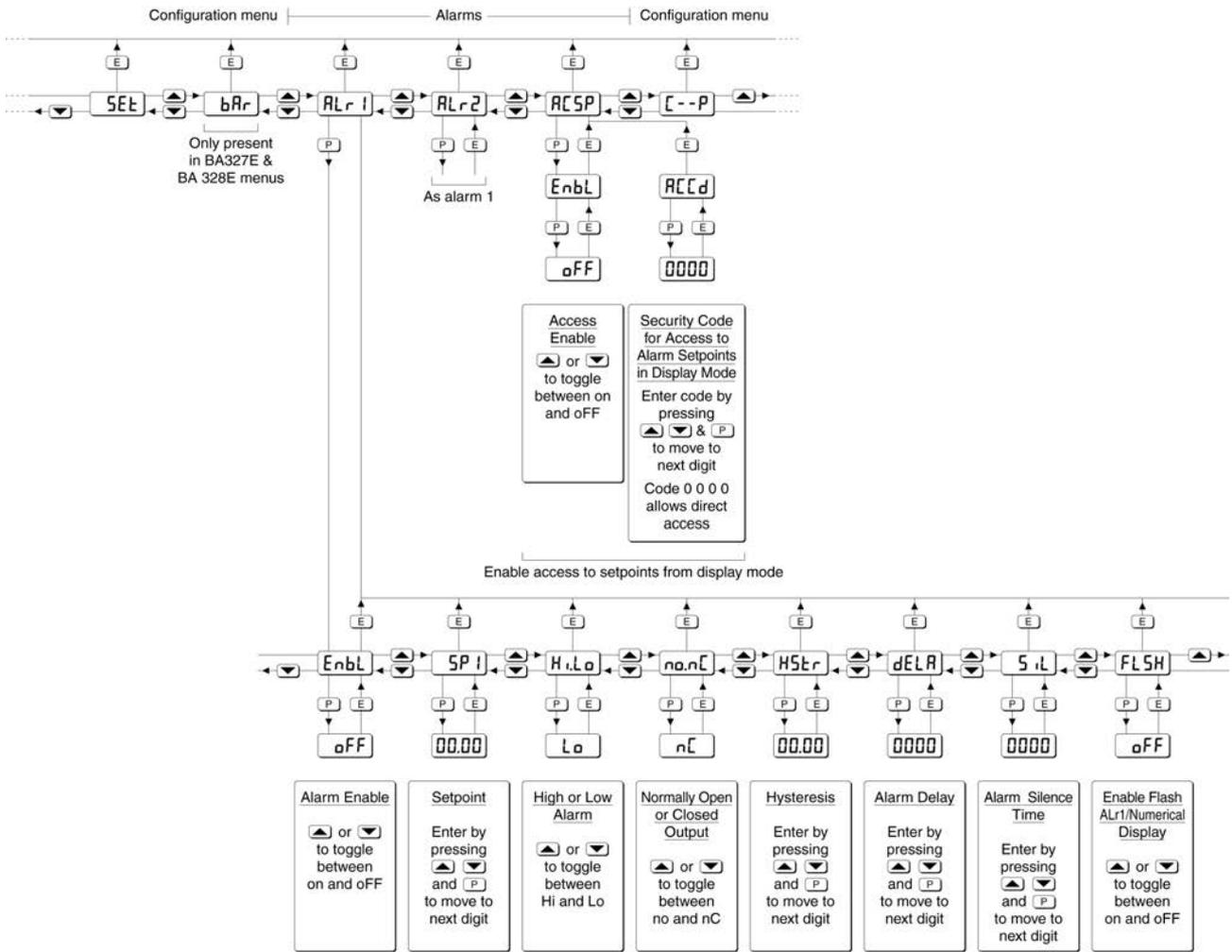
Fig 12 Alarm Configuration Functions in Configuration Menu
