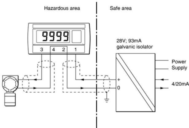
Fig 2b Loop powered by a galvanic isolator
