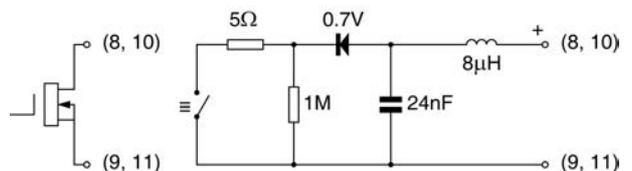
Fig 11 Equivalent circuit of each alarm output
