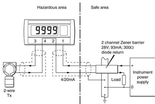
Fig 2a Loop powered by a Zener barrier
