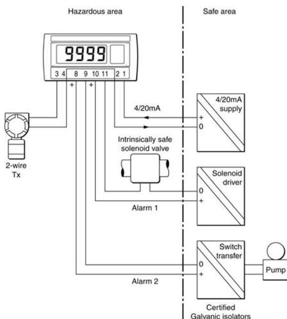
Fig 13 Typical alarm application
