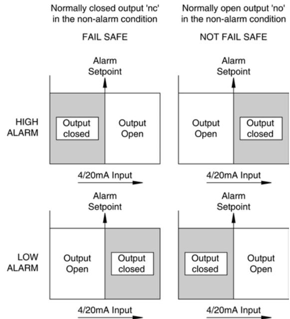
Fig 10 Alarm outputs
