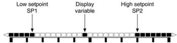
Fig 15 Displayed value and setpoints on bargraph
