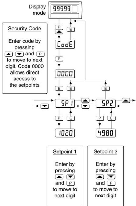
Fig 14 Setpoint adjustment from the display mode
