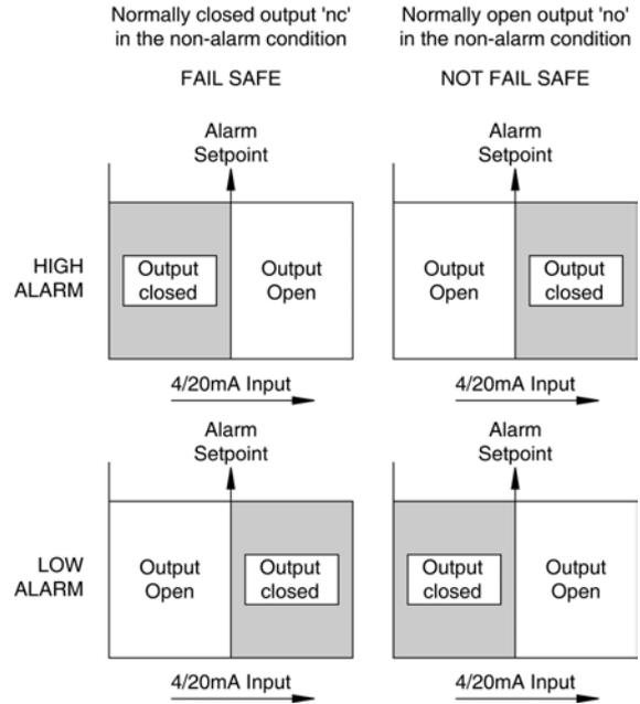
Fig 10 Alarm outputs
