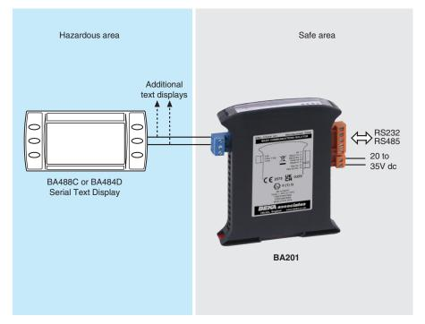
The BA201 communications isolator is a dedicated interface for connecting intrinsically safe BEKA Serial Text Displays to a safe area computer system. The isolator provides intrinsically safe galvanic isolation between the safe and hazardous areas, plus conversion of the RS232 or RS485 safe area serial data to the dedicated communications signalling required by BEKA Serial Text Displays.
