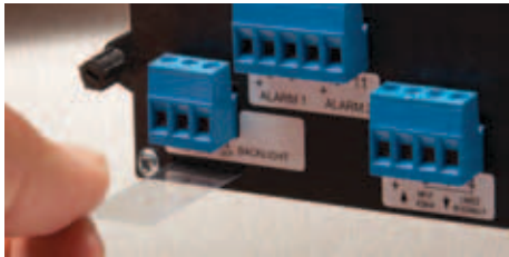
Scale card for 'E' suffix instruments is inserted from the rear of the instrument.
