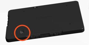
2. Take off the battery cover by pulling on the lid carefully – specifically on the corner with the slant.
