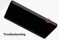
In case device freezes and you need to do a hard reset, **press and hold the power button** for approx. 14 seconds. Device will be turned off now.
