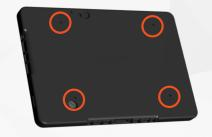
Then replace the 4 corner hex screws of the battery cover using the provided hex tool. The recommended torque for the screw is 10-12Ncm.
