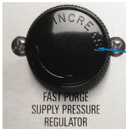
Figure F-11 Fast Purge Supply Pressure Regulator
