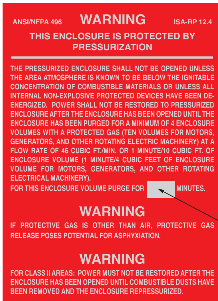
Figure F-1 Warning Label to be installed on the enclosure in a readily visible location (Label included in the AFP-03 installation kit)
