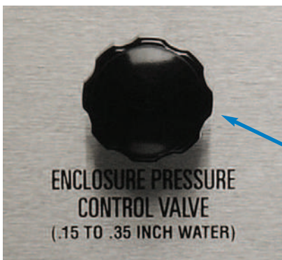
Figure F-16 Enclosure Pressure Control Valve
