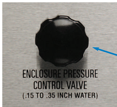
Figure F-10 Enclosure Pressure Control Valve
