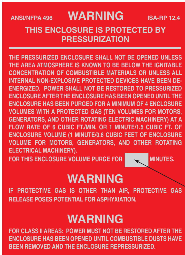
Figure F-8 Warning Label to be installed on the enclosure in a readily visible location (Label included in the AFP-01 installation kit)
