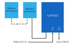
Up to three iUPS101 systems with AC inputs and outputs in parallel with either one or two batteries in series
